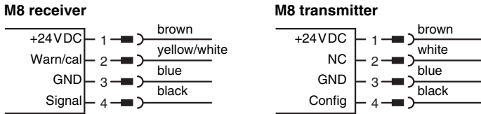
Figure 4.2: Pin assignment of the M8 connector of the VARIO B light curtain
